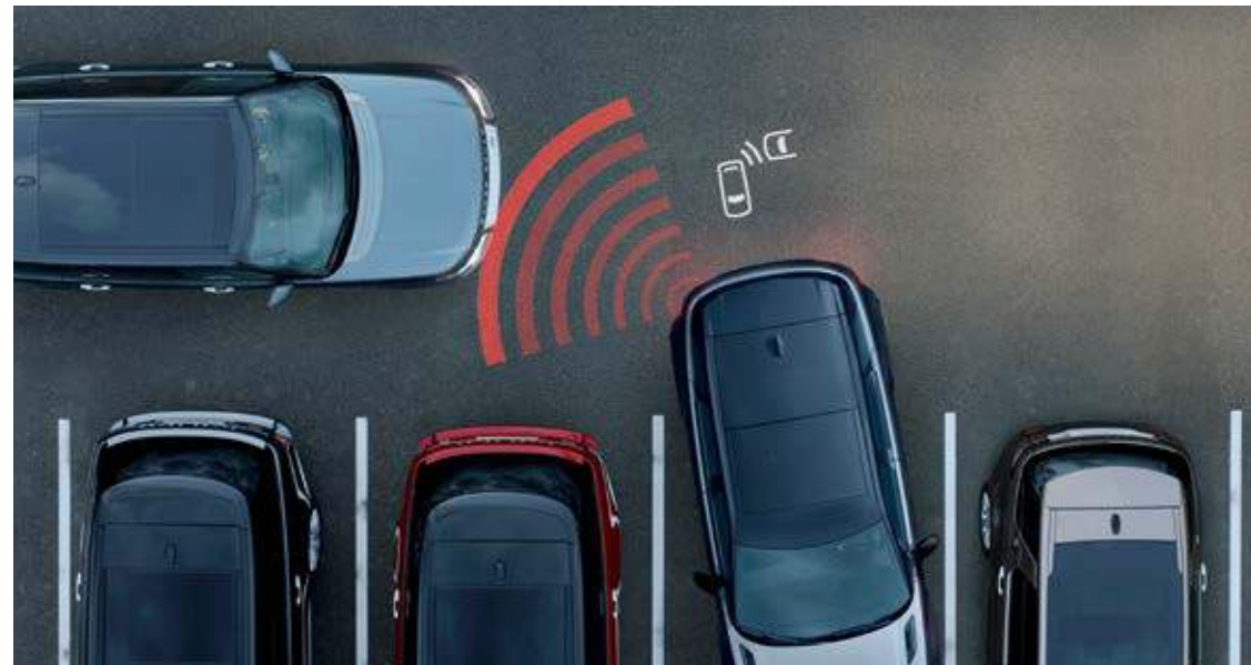
Rear Traffic Monitor
